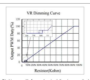
(N=driver quantity for synchronized dimming operation)
