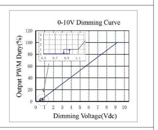
Applying additive PWM signal (Duty: 0- 99%, frequency range 0.25KHz ~ 2KHz, Voltage amplitude: 3-10V)
